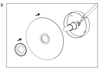
Place the cover plate and ring over the thread.
