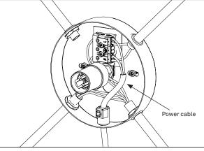
If the cable is surface mounted, put the power cable through the strain relief. Tighten the set screw after pulling the appropriate length through.
