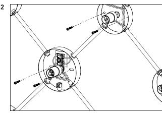
If the lamp is mounted over a junction box, then lead the cable in through the back before proceeding.
